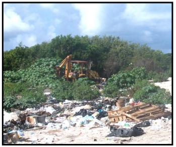
Photo 118. Backhoe used to pile waste up so it can be burned.
