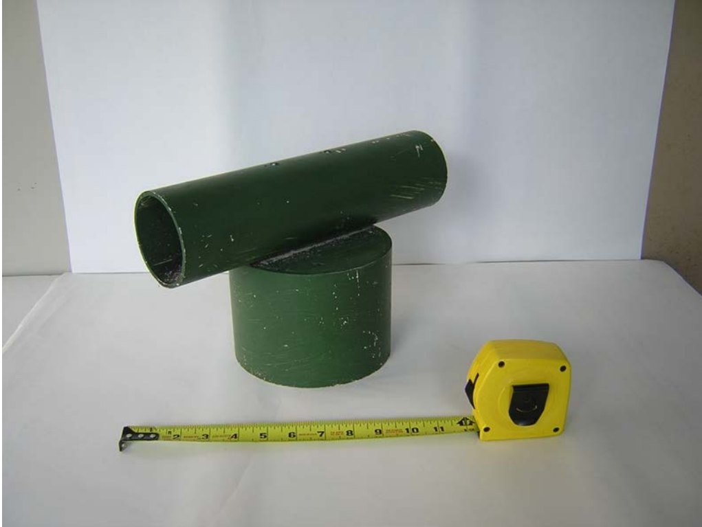
Photo#1: Proposed new bait station constructed of PVC pipes.
