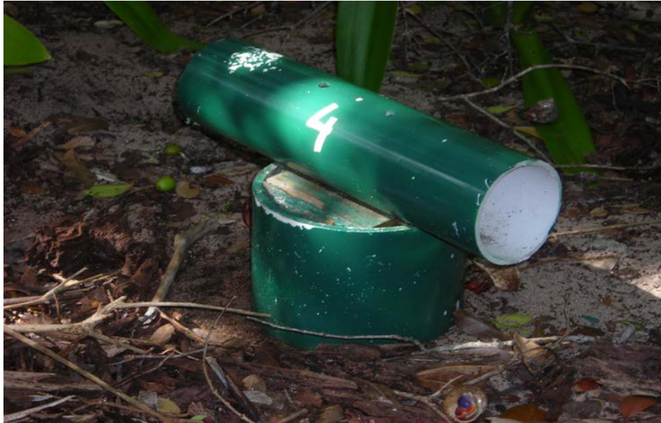
Photo#1: New bait station #4 constructed of PVC pipes.
